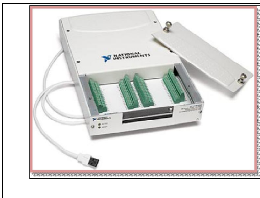
Fig. 4. Data Acquisition card (NI USB-622x M Series)
